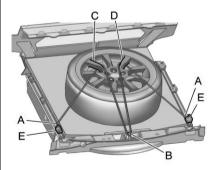
Route one of the hooks (A), at the end of the cable provided, through the liftgate striker (B).
